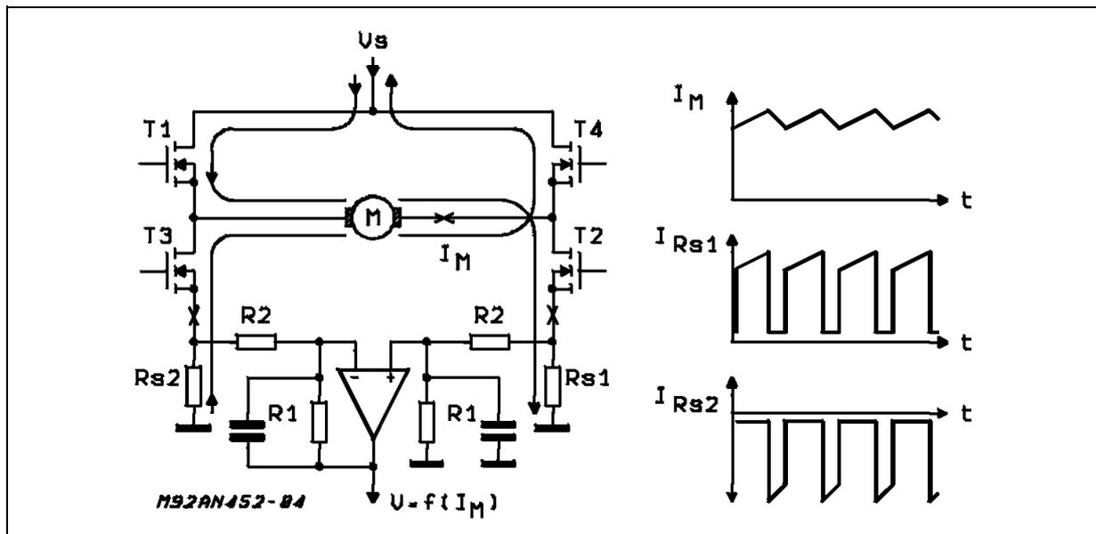
Figure 5. Current Sensing in the Load Circuit.
