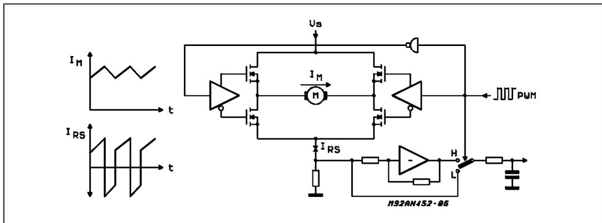
Figure 7. Accovery of the Load Current Map. (Inverting/non Inverting Solution)
