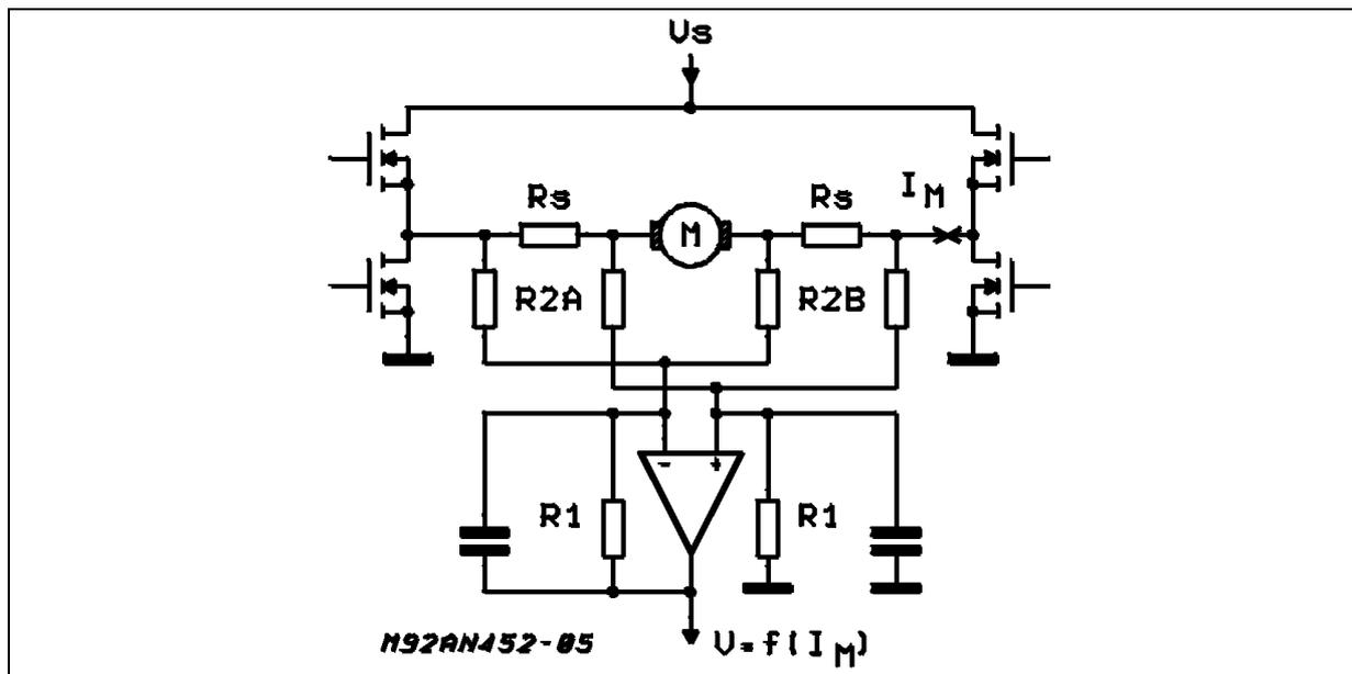
Fig. 5 shows another circuit that is feasible for all situations in which, since they cannot be inserted in the source circuit, the shunts have to be connected directly in series with the load, with all the disadvantages that this entails.
