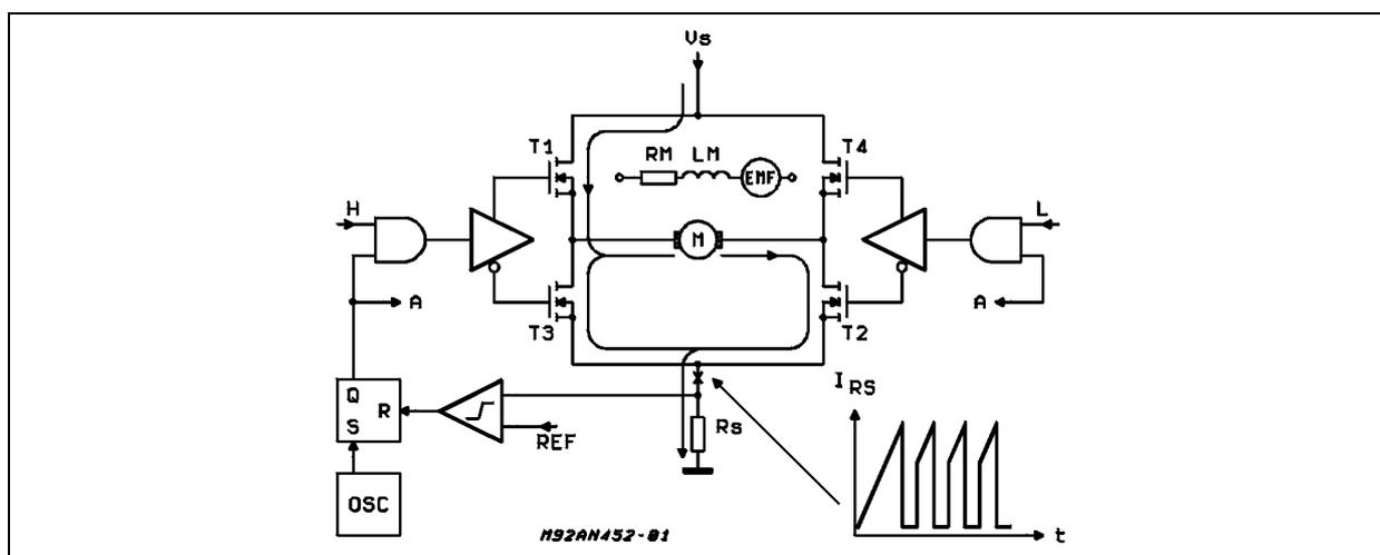
Figure 2. Switch Mode Current Control Circuit for Load Current Limitation.(Bipolar Bridge Configuration)
